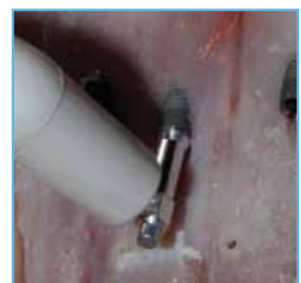
CBCT images showing [a] ideal implant position and available bone height and [b] implant insertion angle [c] acrylic guide secured to a bone specimen to guide drills into the bone under a 20 degrees angle. [d] for implant stability measurements, Osstell Mentor device with suitable SmartPeg was attached to the implant, and RFA was conducted.
